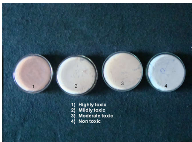
Fig. 1. Toxicity by ammonia vapor test
