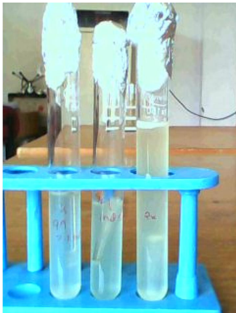
Fig. 9. Presumptive Coliform Test (Acid and gas production)
