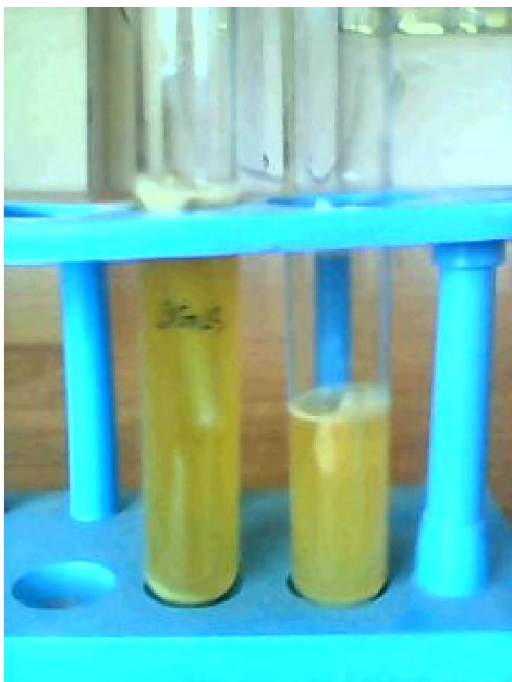
Fig. 9. Confirmed Coliform Test (Gas production)
