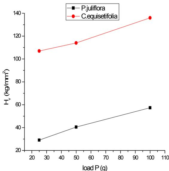
Figure 1. Variation of Vickers micro hardness number  $H_v$  with load
