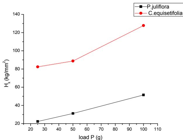
Figure 4. Variation of Knoop micro hardness number  $H_k$  with load
