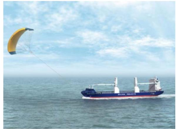
With kite area of 500 m<sup>2</sup> and angle of incidence ranging from 0 to 50 degrees in steps of 5 deg, the lift, drag and total aerodynamic forces are calculated using the following formulas:
