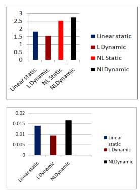
Fig.4. Demand-Capacity ratio and Roof displacement for central column remove
