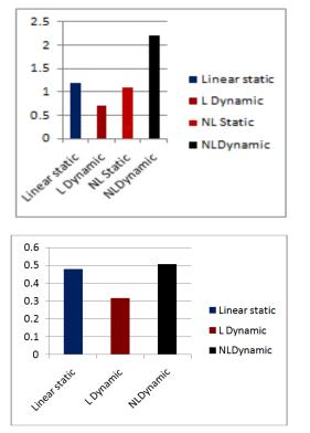
Fig.6. Demand-Capacity ratio and Roof displacement for column of transverse direction remove
