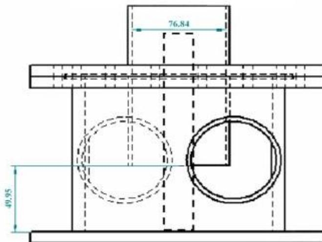
Figure 15. Gap of  $\sim 50.00$  mm between baseplate and nozzle extension used to define the flashback of the system
