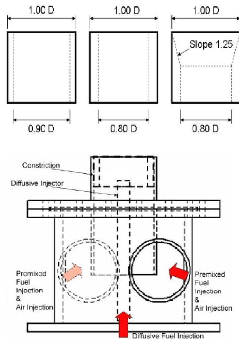
**Figure 3. Diagram of Constrictions and Rig for experimental purposes**
