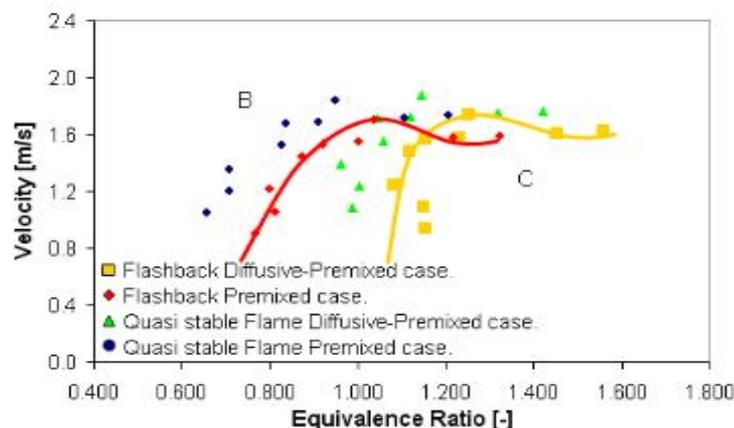
Figure 16. Different regions recognised in the flashback map at atmospheric conditions. B) Region of quastability for the flame, with different flame shapes. C) Flashback region. Region A) Blowout occurs at much lower  $\phi$  and is not visible here
