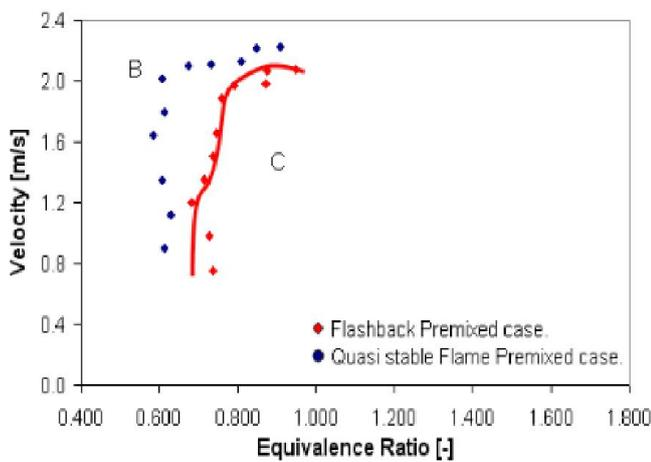
**Figure 17. Different regions in the flashback map at atmospheric conditions using the Quarl Nozzle without fuel injector. B) Region of quasi stability for the flame, with various flame shapes. C) Flashback region**
