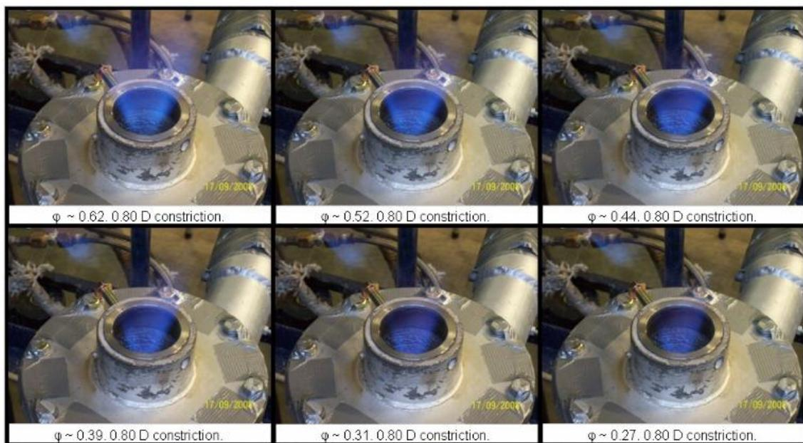
**Figure 12. 0.80 D square constricted case at different equivalence ratios. Gas Injection of 25 l/min diffusive (Wide Injector), 40 l/min premixed**
