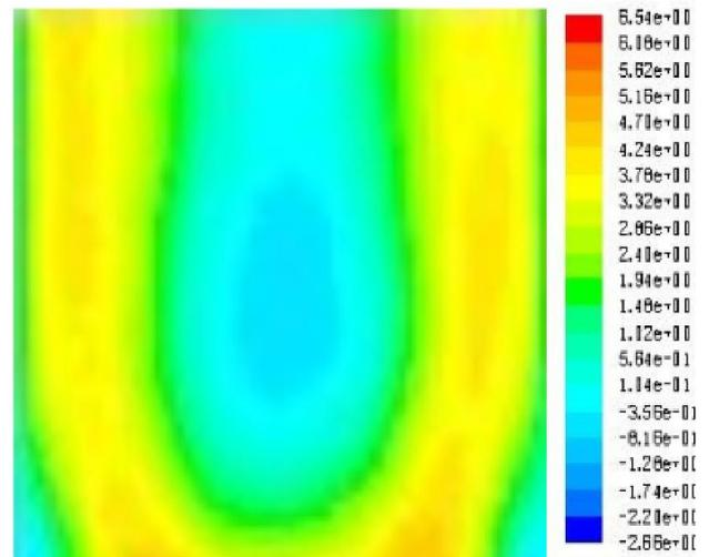
**Figure 19. Modelled velocities showing the CRZ surrounded by the outgoing shear flow. Scale in m/s**
