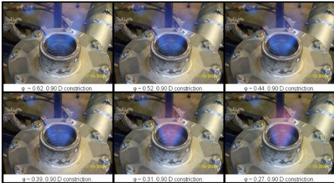
**Figure 11. 0.90 D Tubular exhaust nozzle at various equivalence ratios. Gas Injection of 25 l/min diffusive (Wide Injector), 40 l/min premixed**
