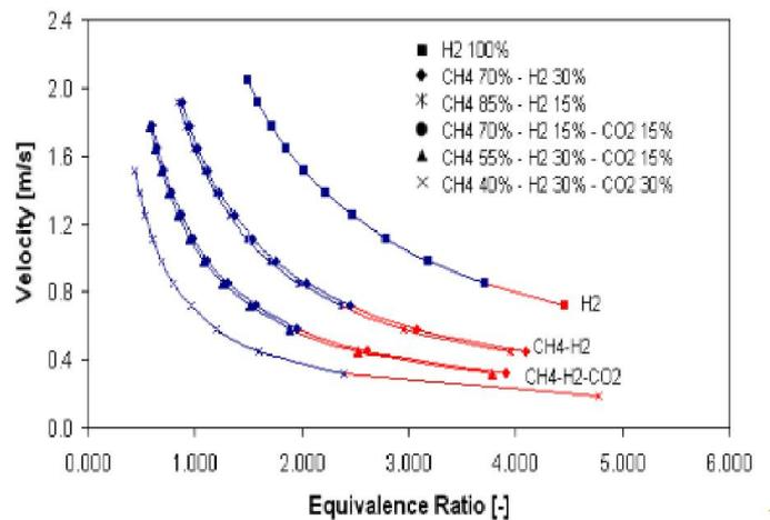
**Figure 20. Flashback analysis for different blends at 1400l/min air flow using No Exhaust Nozzle Constriction at 25-40 l/min gas injection. Flashback (red) and nonflashback conditions (blue). CH4-H2 blends have almost the same trend, as well as CH4-H2-CO2 at 15% CO2**
