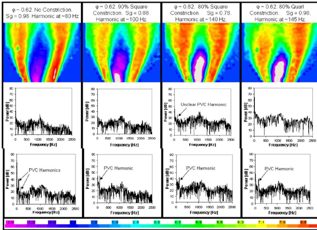
**Figure 14. Combustion at  $\phi \sim 0.62$  and 25-125 l/min gas injection, in comparison with Isothermal case. First row of FFT signals refers to combustion condition. Second row is the Isothermal condition. A) Non-confined. B) 0.90D square confinement. C) 0.80D Square confinement. D) Quarl Confinement. The colour bar represents the flow velocity (m/s), with colour white being out of the range (extremely strong negative velocity for these cases)**
