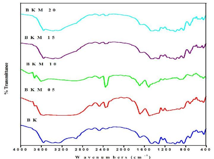
**Fig. 2. Infrared spectra of BKM glasses with different concentration of MgO**
