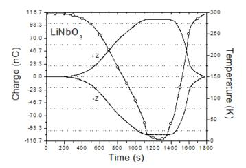
Fig. 3. Temperature of the crystal and the change in polarization charge from the polarization charge at 300K of a crystal of LiNbO $_3$  as functions of time. The curve with the open circles is a plot of the temperature as a function of time. The solid unmarked curves represent the change in the polarization charge relative to that at 300K at the +z base and the-z base of the crystal. The data for the three curves were recorded simultaneously
