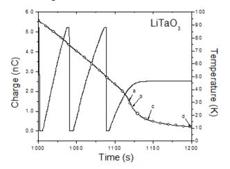
Figure 4B. Expansion of the plots of LiTaO $_3$  around the region of point (c) to include the region beyond point (d) of Fig. 4A, i.e., the interval of time from 1,000s to 1,200s. From point (a) to point (b) the temperature changed from 31.52K to 26.27K and the relative polarization charge changed from 2.12nC to 2.45nC. From point (c) to point (d) the temperature changed from 16.70K to 11.02K and the relative polarization charge changed from 2.52nC to 2.53nC
