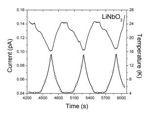
Figure 8B: Expansion of the response of  $LiNbO_3$  in the time interval of about 4,200s to about 6,000s, which shows the polarization current centered at point (b) of Fig. 8A, corresponding to the three smallest temperature cycles. At this large magnification, the breaks in the current are clearly visible.
