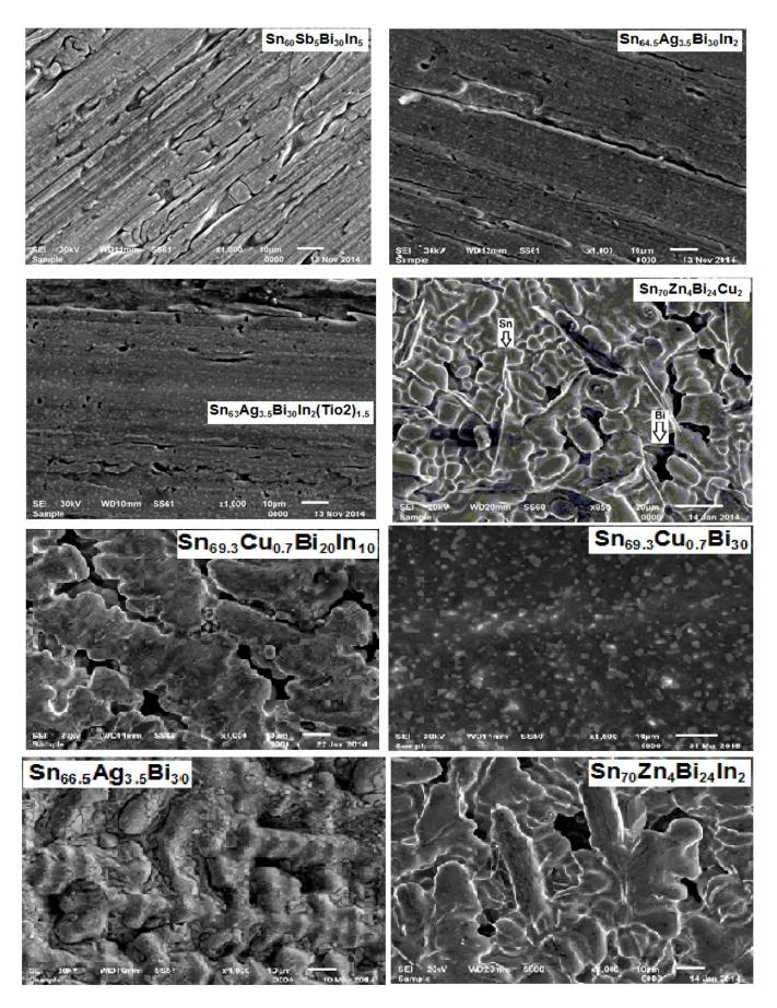
Figure 2. SEM of tin- bismuth based alloys
