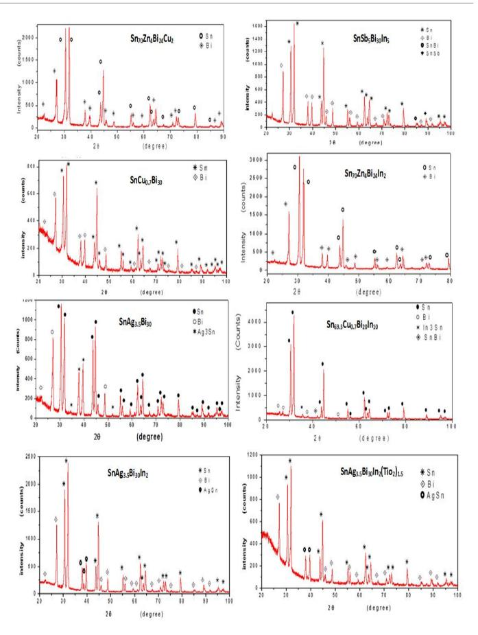
Figure 1. X-ray diffraction patterns of tin- bismuth based alloys
