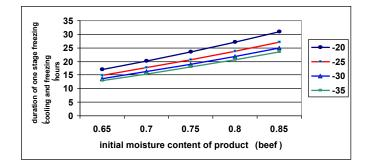
Fig 2. Duration of one stage freezing as a function of moisture content of product (beef) and cooling air temperature
