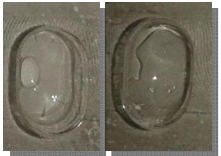
Fig . Drops collapse test, Right: D.W, Left: Pseudomonas fluorescens
