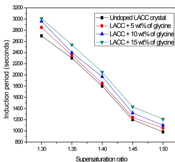
Fig.2. Variation of induction period with supersaturation ratio for undoped and glycine doped LACC samples
