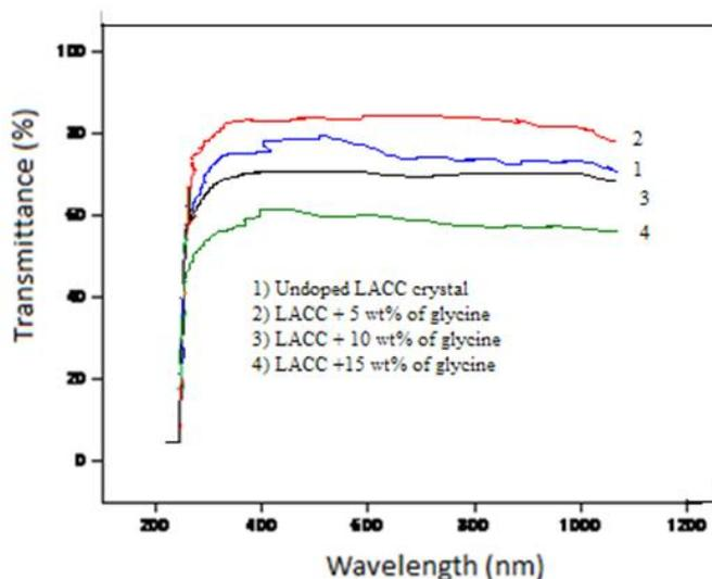
**Figure 8. UV-visible transmittance spectra of undoped and glycine doped LACC crystals**
