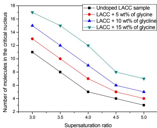
Fig.5. Variation of number of molecules in the critical nucleus with supersaturation ratio for undoped and glycine doped LACC samples
