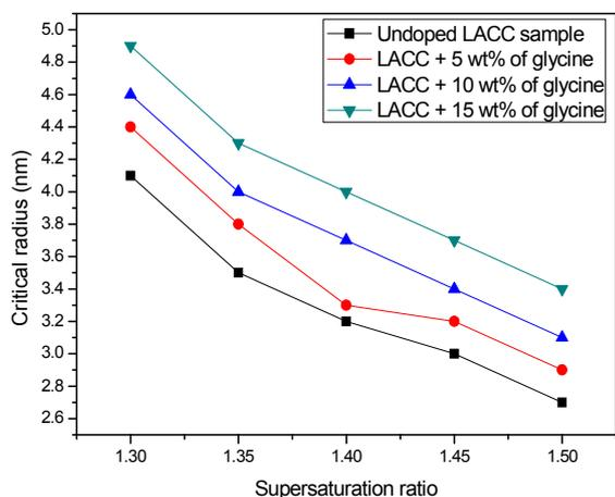
Fig.4. Plots of critical radius with supersaturation ratio for glycine doped LACC samples
