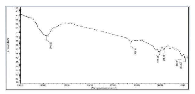
Fig.1. FTIR of surface modified 4 HAOT-II copolymer
