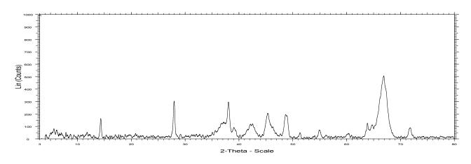
Fig 3. XRD pattern of surface modified 4 HAOT-II copolymer
