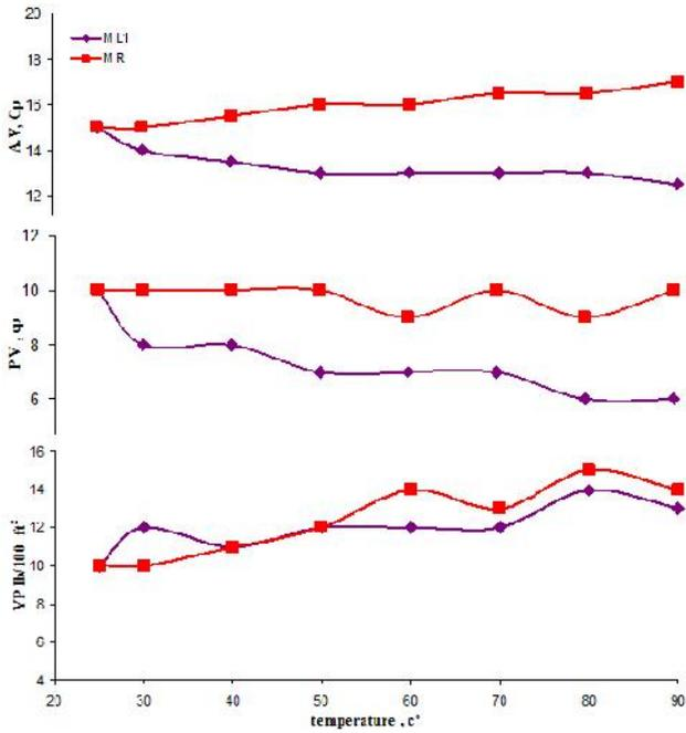
Figure10. Rheological properties of formulated mud ML<sub>1</sub> compared to MR at different temperatures
