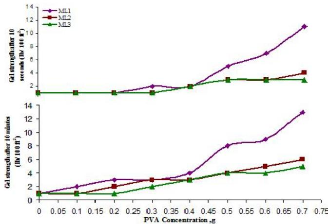
Figure 8.  $G_{10sec}$ ,  $G_{10 min}$ , and concentration of PVA relationship of formulated muds (ML<sub>1</sub>, ML<sub>2</sub> and ML<sub>3</sub>)
