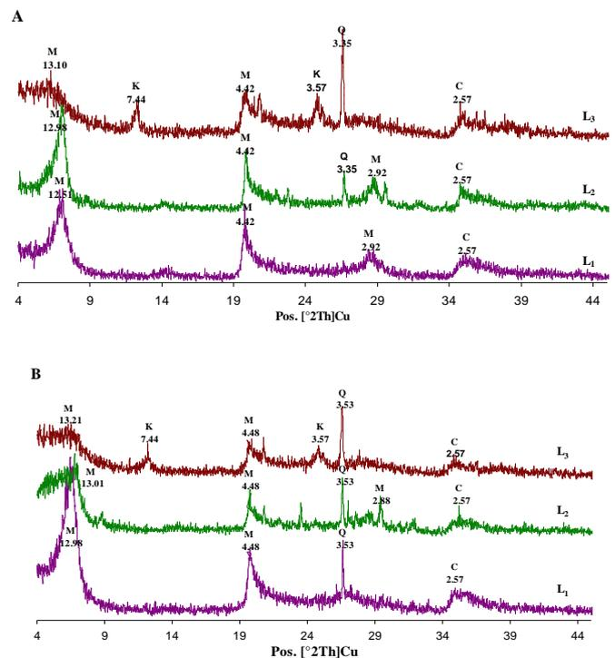
**Figure 1. (A) X-ray diffraction analysis of untreated samples (L<sub>1</sub>, L<sub>2</sub> and L<sub>3</sub>) and (B) for treated bentonite samples (L<sub>1</sub>, L<sub>2</sub> and L<sub>3</sub>) with PVA ( M=Montmorillonite, C= Calsite, K= Kaolinite and Q = Quartz)**
