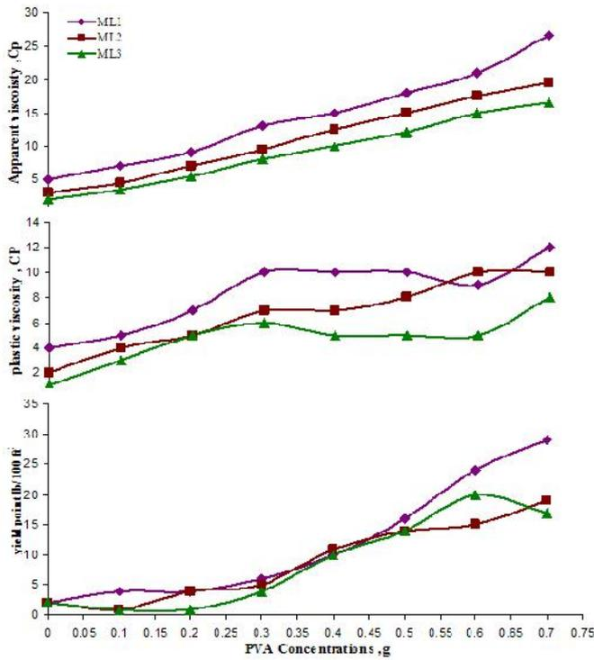
Figure 7. Rheological properties, concentration of PVA relationship for formulated mud batches (ML<sub>1</sub>, ML<sub>2</sub> and ML<sub>3</sub>)
