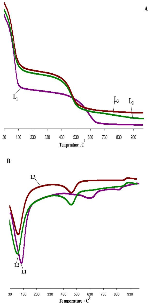
Figure 2. TGA for Fig. (A) and DTA for Fig. (B) For local untreated bentonite samples  $L_1$ ,  $L_2$  and  $L_3$
