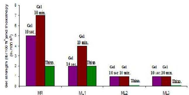
Fig 6. Gel strength after 10 sec. and after 10 min. and thixotrop for  $ML_1$ ,  $ML_2$  and  $ML_3$  before activation with PVA compared with MR
