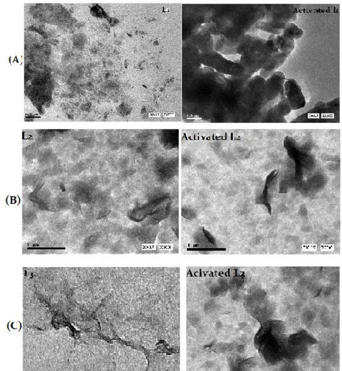
Figure 4. TEM micrograph of (A) row  $L_1$  and activated  $L_1$ , (B) row  $L_2$  and activated  $L_2$  and (C) row  $L_3$  and activated  $L_3$
