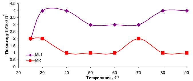
Figure 12. Temperature relationship, Thixotropy of formulated mud ML<sub>1</sub> compared to MR
