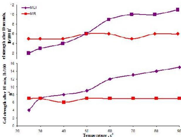
Figure 11. Temperature relationship, Gel strength of formulated mud ML<sub>1</sub> at 10 sec. and 10 min. compared to MR
