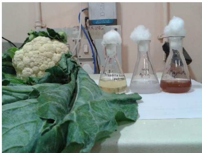
Fig. 1. Cauliflower leaves, 5% v/v Brassica oleracea L extract, 1mM silver nitrate solution and silver nanoparticles with reddish brown colour
