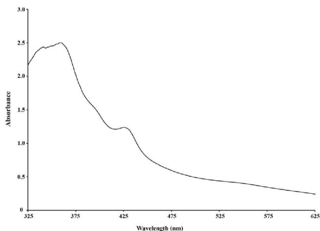
Fig.3. UV-Visible Spectra of the synthesized AgNPs
