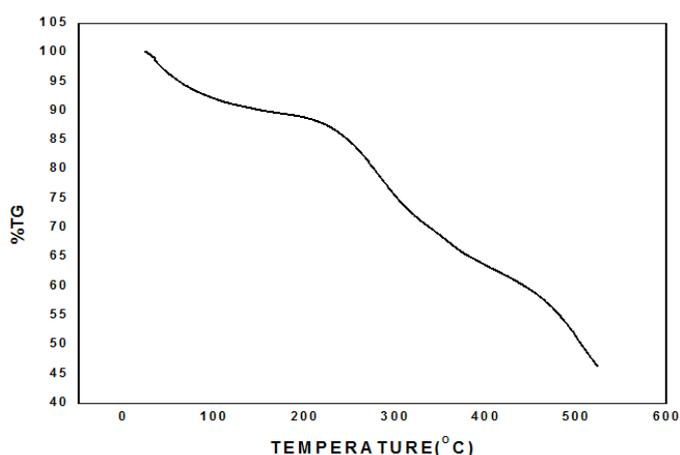
Fig. 11. TG curve of the AgNPs at different temperatures
