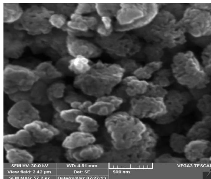
Fig.5. SEM image of AgNPs using CRGE leaf extract
