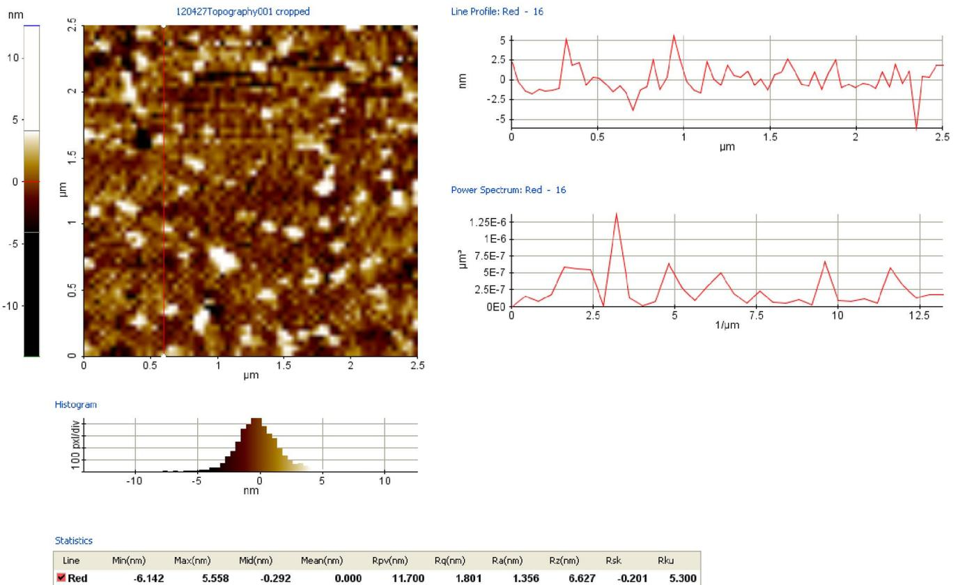
**Fig. 9. AFM size distribution image of AgNPs**
