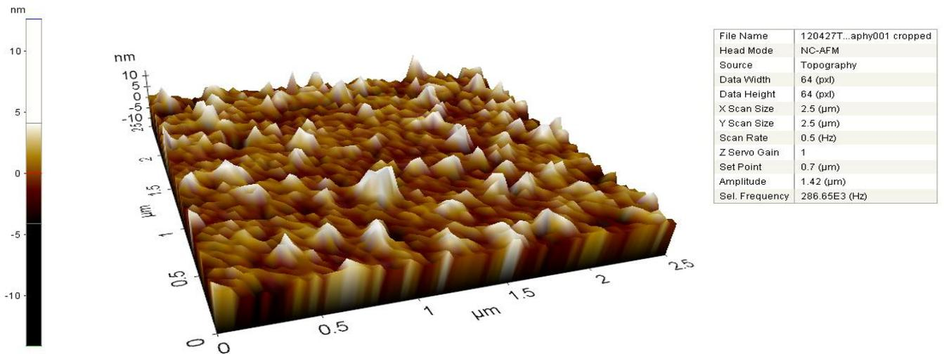
**Fig. 8. AFM topographical image of AgNPs**
