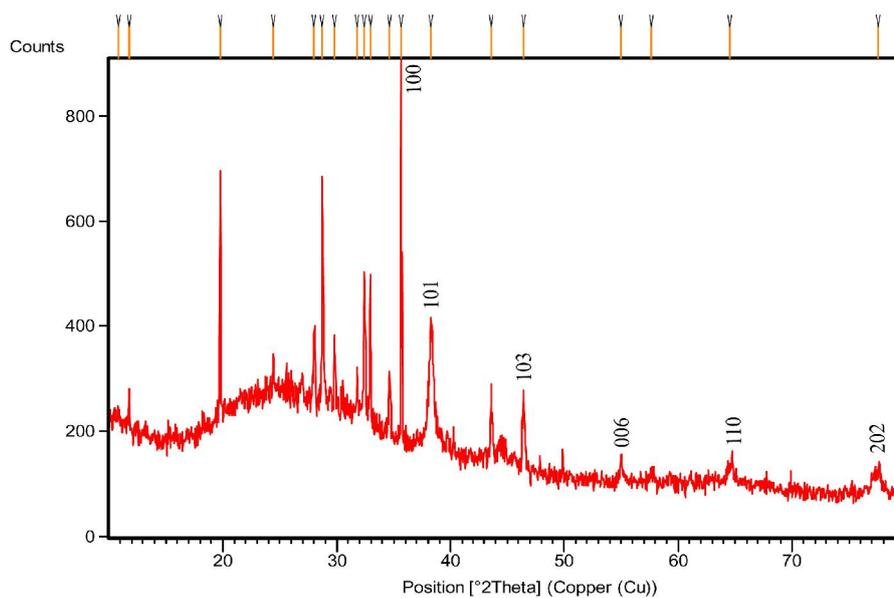
Fig. 7. X-ray diffraction pattern of AgNPs
