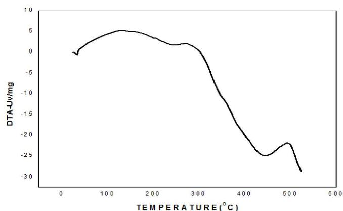
Fig. 12. DTA curve of the AgNPs at different temperatures
