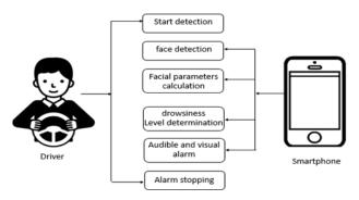
This is the representation of system that how it will work. The drowsiness detection application present in mobile will start the facial detection, it will determine the level of drowsiness and then it will fire an audible alarm which will help to alert every one present in the vehicle. We were connecting the mobile with Bluetooth which will increase the volume of alarm.
