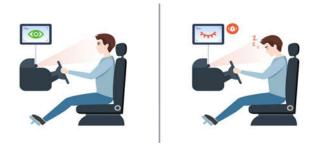
As we can see in above image the device or mobile containing driver drowsiness detection application will be placed in front if driver, on the steering which will continuously read the face of driver and watch the eyes of driver, if eyes get close it will fire the alarm immediately.
