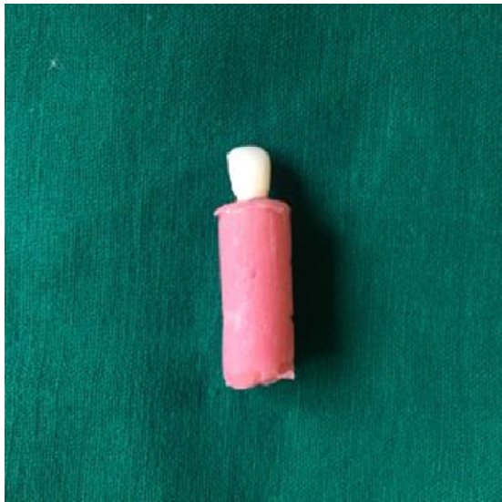
Figure 1. Roots embedded in self-cure acrylic resin
