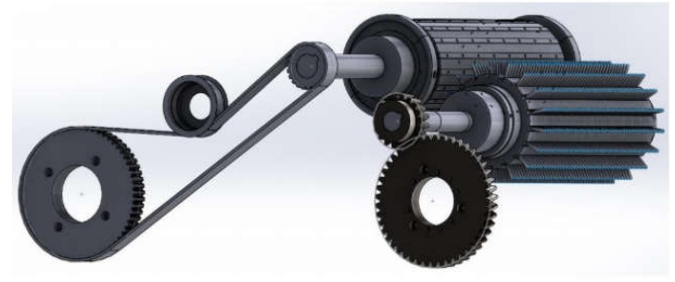
Fig. 3. General picture of the working principle of the combing machine
