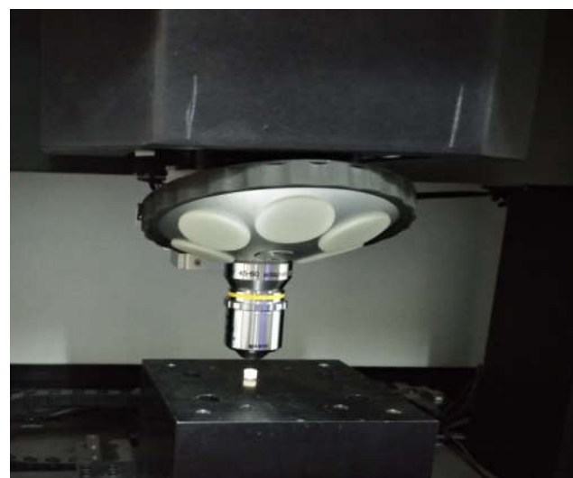
Figure 3. Measurement of surface roughness
