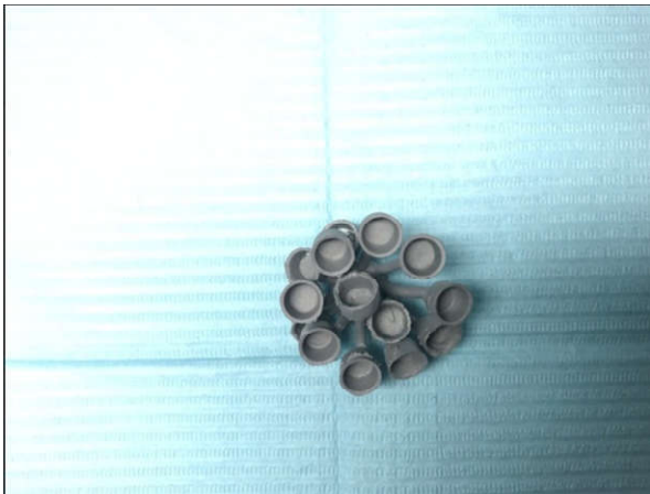
Figure 5. Casted crowns before removing of sprues
