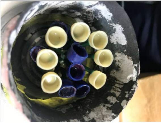
Figure 4. Manufactured wax patterns in the casting ring before investment
