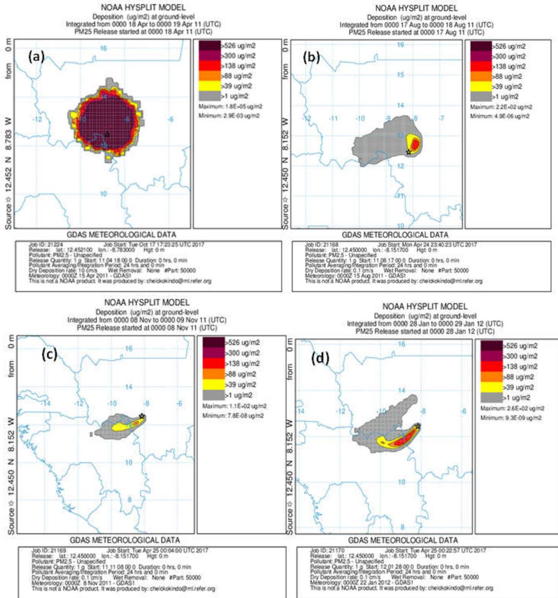
Figure 4. Simulated PM<sub>2.5</sub> particle deposition over 24 hours (a) from 18 to 19 April 2011 (b) from 17 to 18 August 2011 (c) from 08 to 09 November 2011 and (d) from 28 to 29 January 2012
