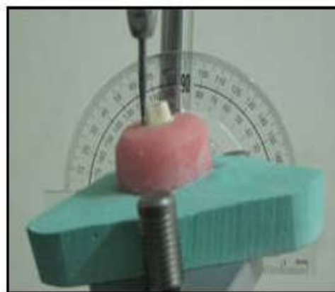
Figure 2. Mounted tooth assembly on platform of milling machine tilted to achieve convergence of 20 degrees
