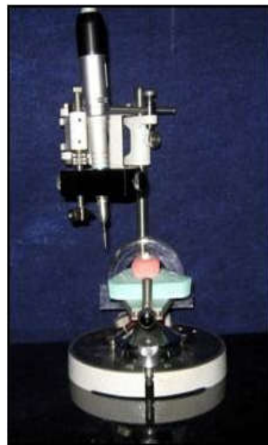
Figure 1. Milling machine attached with a hand piece and mounted tooth assembly for preparation of teeth
