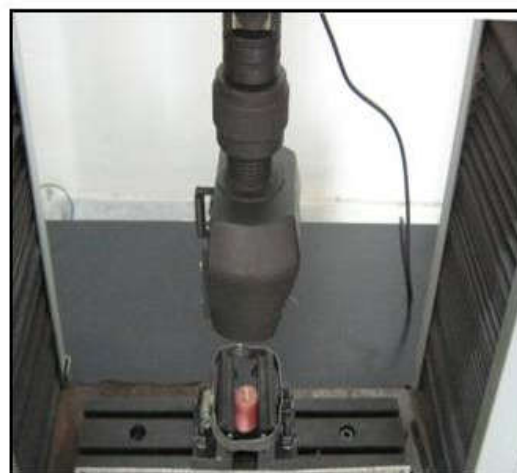
Figure 3. Wire passed through hole in the coping and attached to the upper apparatus of the Universal Testing Machine
