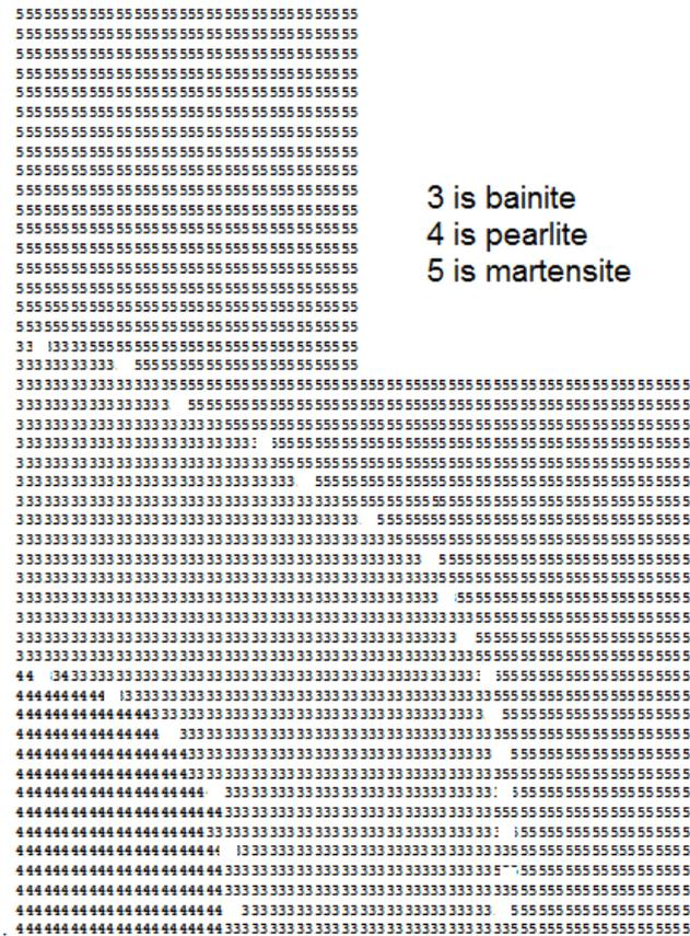
Fig. 7 Micro – structure distribution in a small roller at the moment of time 70 sec when quenched in condition Kn = 1: 3 is bainite, 4 is pearlite, 5 is martensite.
