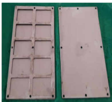
Fig. 1a. Fabricated molds for flexural strength
