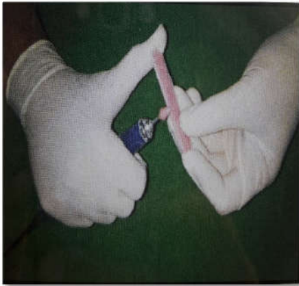
Fig. 13. Finishing of the specimens
