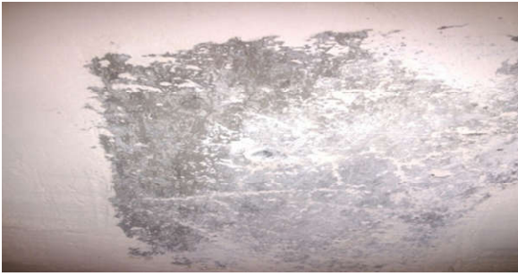
Fig. 9. Bullet test do not penetrate instead just caused a minor dent
