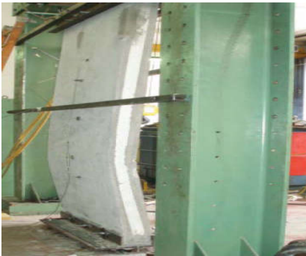
Fig. 11. Compression test result in bending at 700 KN
