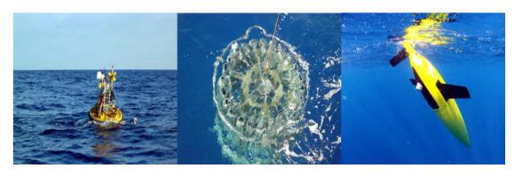
Figure 2. A weather-oceanographic Dolan buoy (left), water sampling rosette (centre), autonomous underwater vehicle glider (right)
