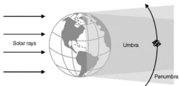
Figure 3. Umbra and Penumbra [Source: Satellite Communications. Authors: Anil Kumar Maini, Varsha Agrawal, Originally published: April 2010]
