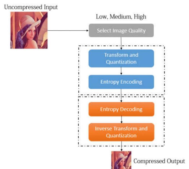
Fig. 2. Architecture of Image Compression
