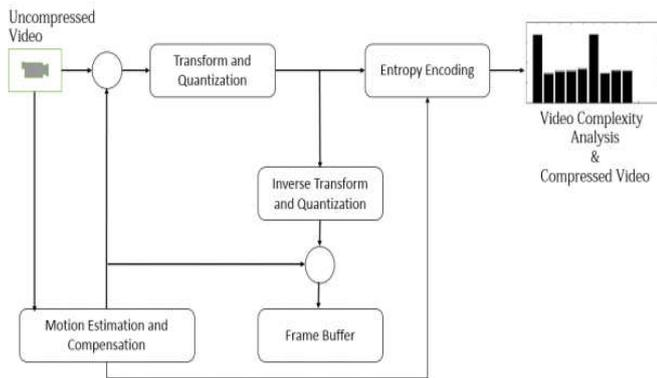
Fig. 3. Architecture of Video Compression
