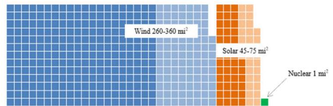
**Figure 10. Comparison of 1000 MW nuclear with wind and solar power plants which can produce the same power annually (nuclear energy institute, 2015)**
