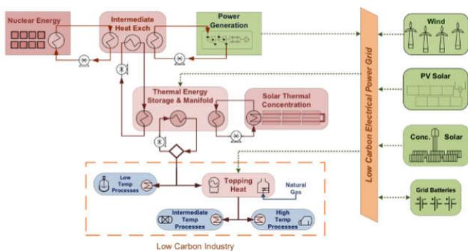
**Figure 6. General architecture for a thermally coupled nuclear renewable hybrid energy system, developed by: Idaho National Laboratory (US DOE, 2015)**
