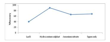
Figure 1. Effect of modifying agents on Pb atomic absorption signal using 1% modifyer agent
