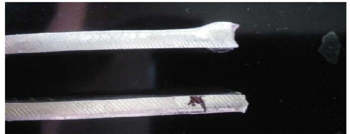
**Figure 1. Failed tensile test specimen showing cup and cone type fracture**
