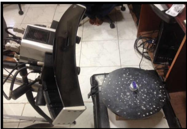
Fig.7. 3D scanner (Solnix, Rexscan-3, Germany)
