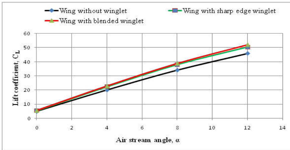
Figure 4. The distribution of the Coefficient of lift against air stream angle ( \alpha ), for different wing shapes
