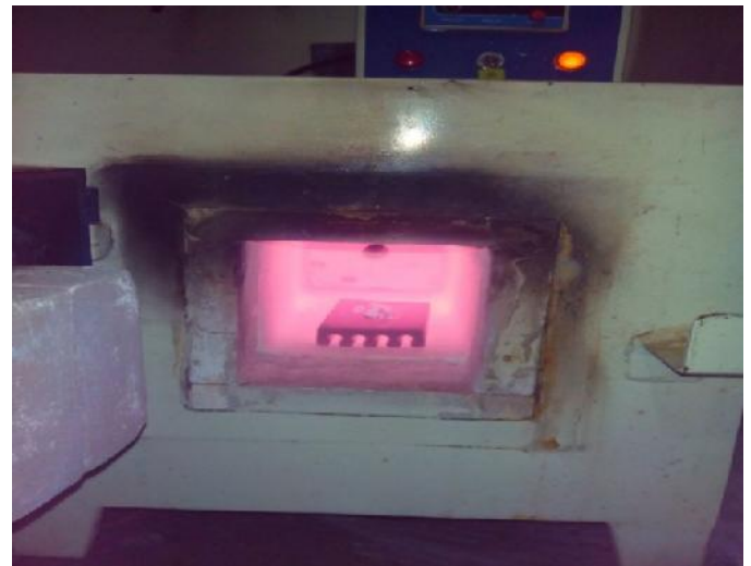
Fig. 2. Ceramic brick containing teeth placed in the furnace
