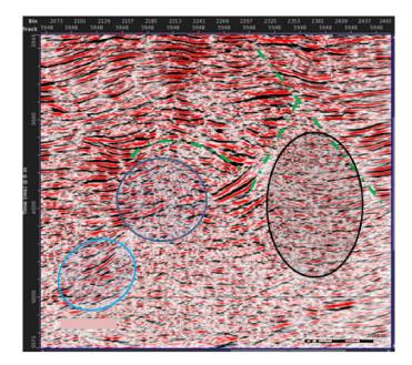
Fig. 5. 3d PSDM section after detailed velocity analysis as applied in this study; event continuity is enhanced within the circled zones; Fault lines are clearer and a rollover strucure becomes more identifiable than in the previous section
