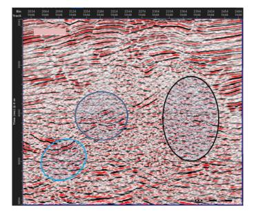
Fig. 4. 3d PSDM section Prior to Detailed velocity analysis as applied in this study; beyond 3000ms, reflection events are indiscernible, fault lines and structures are unidentificable
