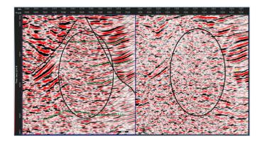
Fig. 6. Comparison of areas at the footwall of the fault; Observe the chaotic nature of reflection eventswithin the circled zone in B; Events are more continious in the corresponding circle in A - (illustrated by the green dotted lines in A)
