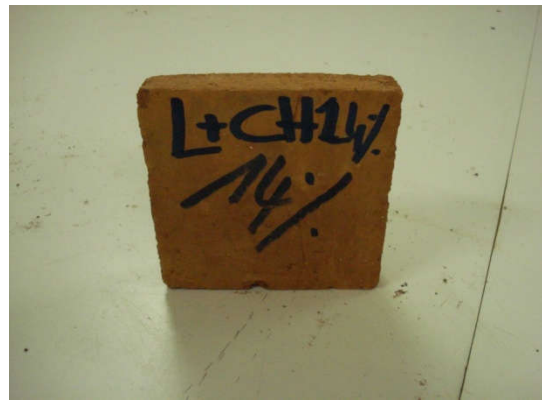
Figure 2. Image of a laterite brick plus 14% of lime
