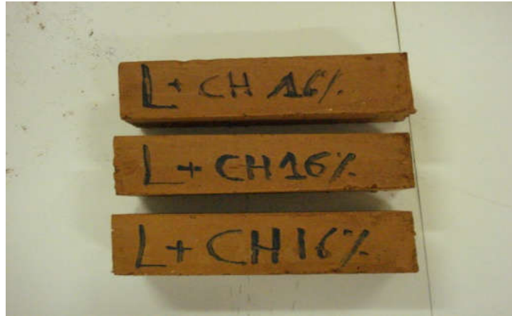
Figure 6. Test tubes for mechanic tests (laterite plus 16% of lime)
