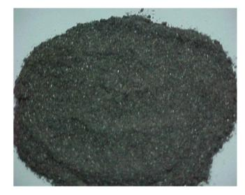
Figure 7. Ash Particle Size Less than 0.5 mm
