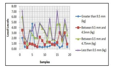
Figure 13. Samples Vs. Lead Concentration as in EP Toxicity Test
