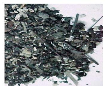
Figure 8. Ash Particle Size between 0.5-4.75 mm
