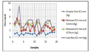
Figure 12. Samples Vs. Zinc Concentration as in EP Toxicity Test
