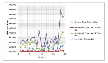
Figure 4. Lead concentration in ash
