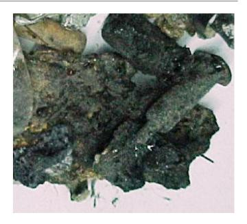
Figure 10. Ash Particle Size Greater than 9.5 mm
