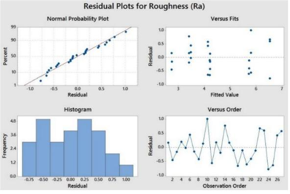
Fig. 2. Residual plots for roughness of HCHCR
