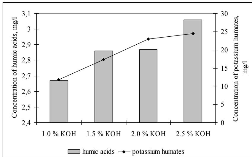
Figure 2. An extractant concentration effect on the quality of the liquid Humic fertilizer
