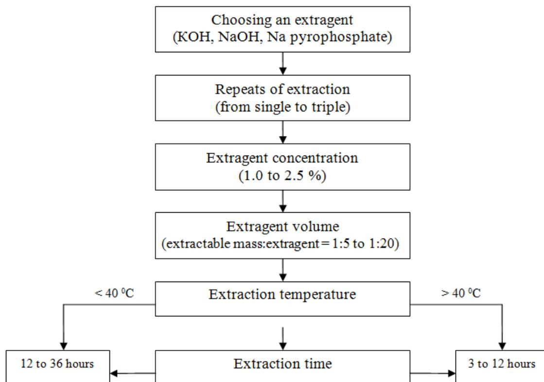
Figure 1. An algorithm for production of a liquid Humic fertilizer from biotechnological production wastes
