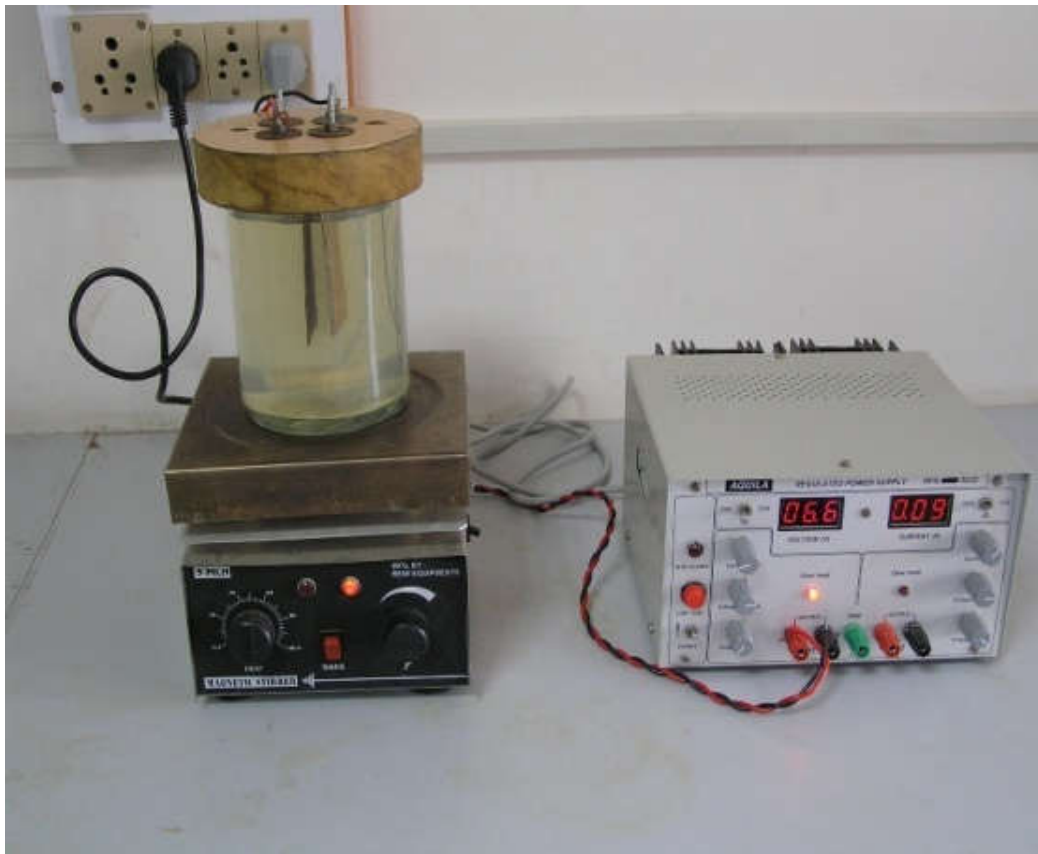
Figure 1(a). Laboratory bench-scale Electro coagulation set-up
