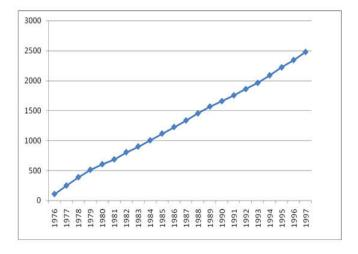
Figure 3: Mass curve using data from Kisumu Airport meteorological station
