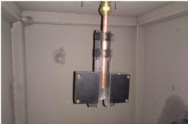
Figure 7. Device for measuring particle velocity
