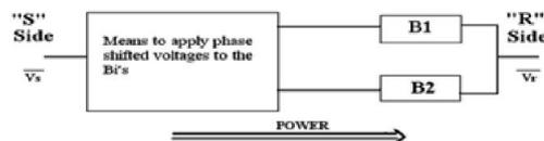
**Fig. 1. Single line diagram of principle IPC**
