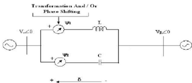
**Figure 1. Operating Principle of IPC**
