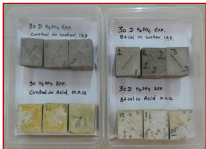
Fig.4. Control and Bio-admixture incorporated specimens showing residual alkalinity after 30, 60, 90 days in HCl and H 2 SO 4
