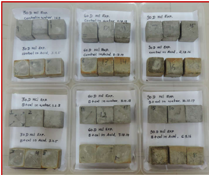
Fig.2. HCl exposed mortar specimens (with and without Bio-admixture) after 30,60,90 days
