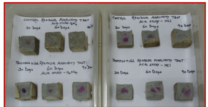
Fig.4. Control and Bio-admixture incorporated specimens showing residual alkalinity after 30, 60, 90 days in HCl and H 2 SO 4
