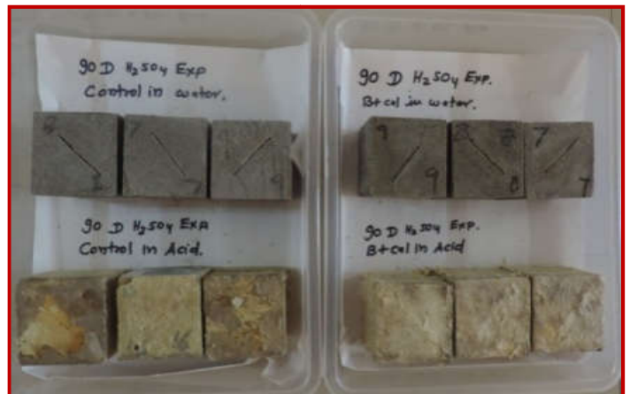
Fig.3. H 2 SO 4 exposed mortar specimens (with and without Bio-admixture) after 30,60,90 days
