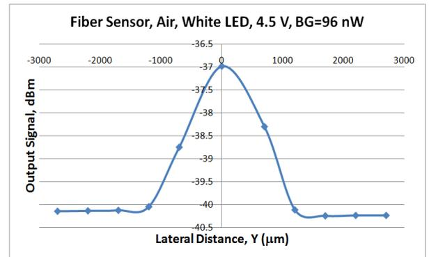
Figure 6. Output power in order of dBm for changing lateral distance of Y axis
