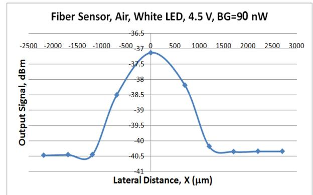
Figure 6. Output power in order of dBm for changing lateral distance of X axis
