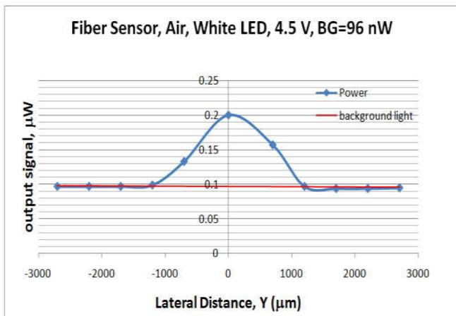
Figure 4. Output power in order of microwatt for changing lateral distance of Y axis
