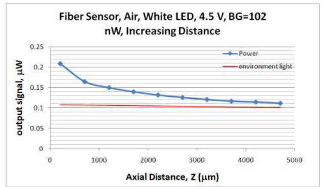
Figure 5. Output power in order of microwatt for changing axial distance of Z axis
