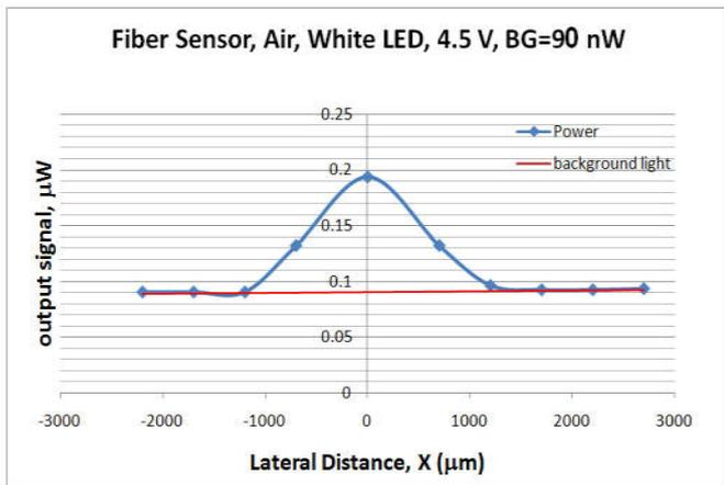
Figure 3. Output power in microwatt for changing lateral distance of X axis
