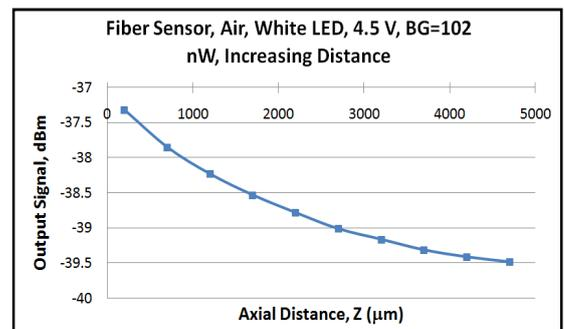
Figure 6. Output power in order of dBm for changing axial distance of Z axis
