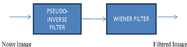
**Fig. 2. Pseudo noise filter and filtered image**
