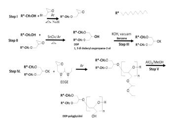
Fig 1. Schematic diagram of the synthesis of DDP-PG DDP-PG was synthesized from the precursor di-dodecanols and with protective glycidol, ethoxy ethyl glycidyl ether (EEGE) followed by a terminal hydrolysis of methanolic AlCl<sub>3</sub>. Chemical structure of the polyglycidol-derivatized lipid, DDP-PG, used in this study. Molecular weight, Mw = 2650, degree of polymerization of the polyglycidol chain, n = 30.
