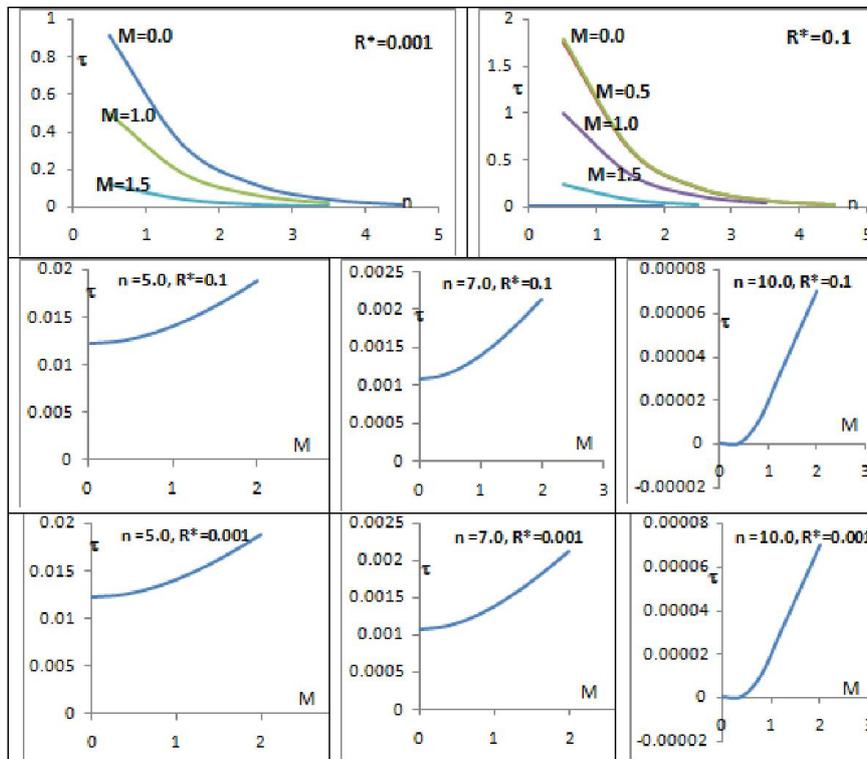
**Fig. 3. Variation of skin-friction with  $n$  and  $M$ , at  $R^*= 0.001$  &  $0.1$**
