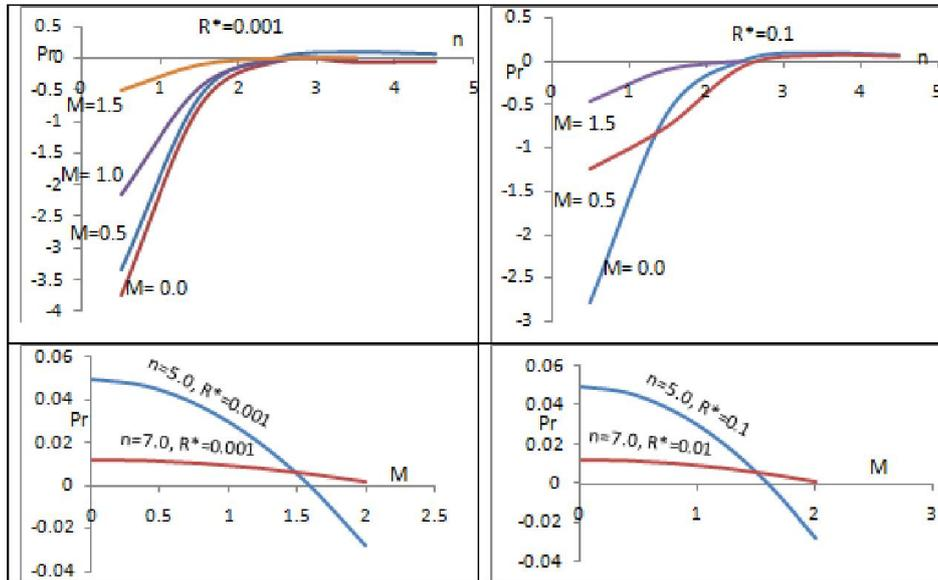
Fig. 4. Variation of Pressure with  $n$ ; for  $M = 0.0, 0.5$ , at  $R^* = 0.1$  &  $0.001$
