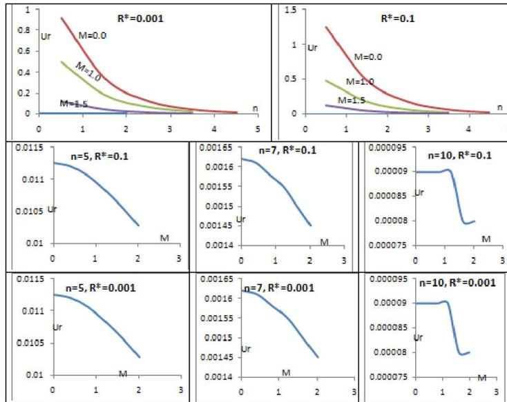
**Fig. 2. Variation of radial velocity with  $n$  &  $M$  at  $R^*=0.001$  &  $0.1$**
