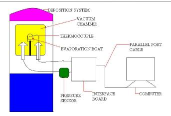
Fig. 4. Schematic diagram of the designed computer based temperature and pressure measuring system tested in Edward auto 306 magnetron sputtering system
