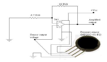
Fig. 1. The designed circuit of the pressure sensor MP20C-01-F2
